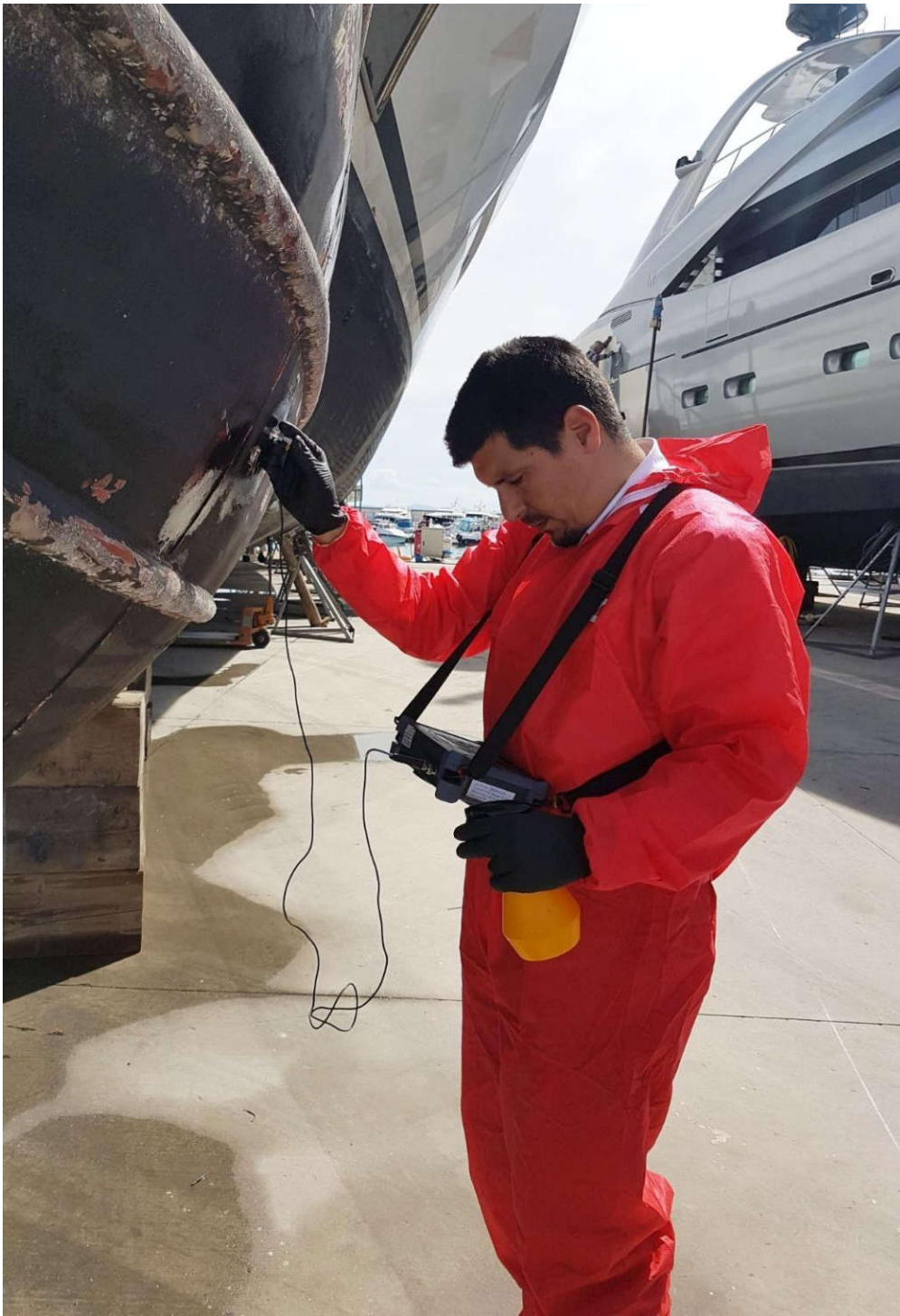
Cem Baykent inspects the hull of a marine vessel using the EPOCH 650 ultrasonic flaw detector
