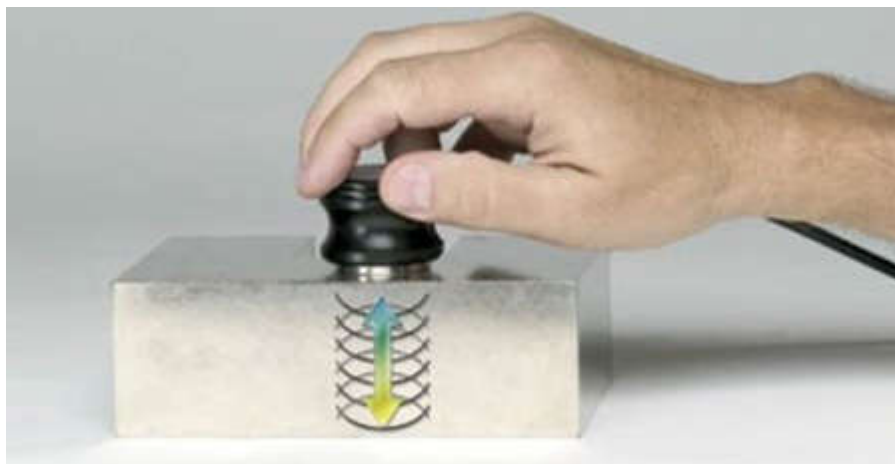
A sound pulse generated by a transducer travels through a test piece and reflects back from the inside (here lower) surface.
