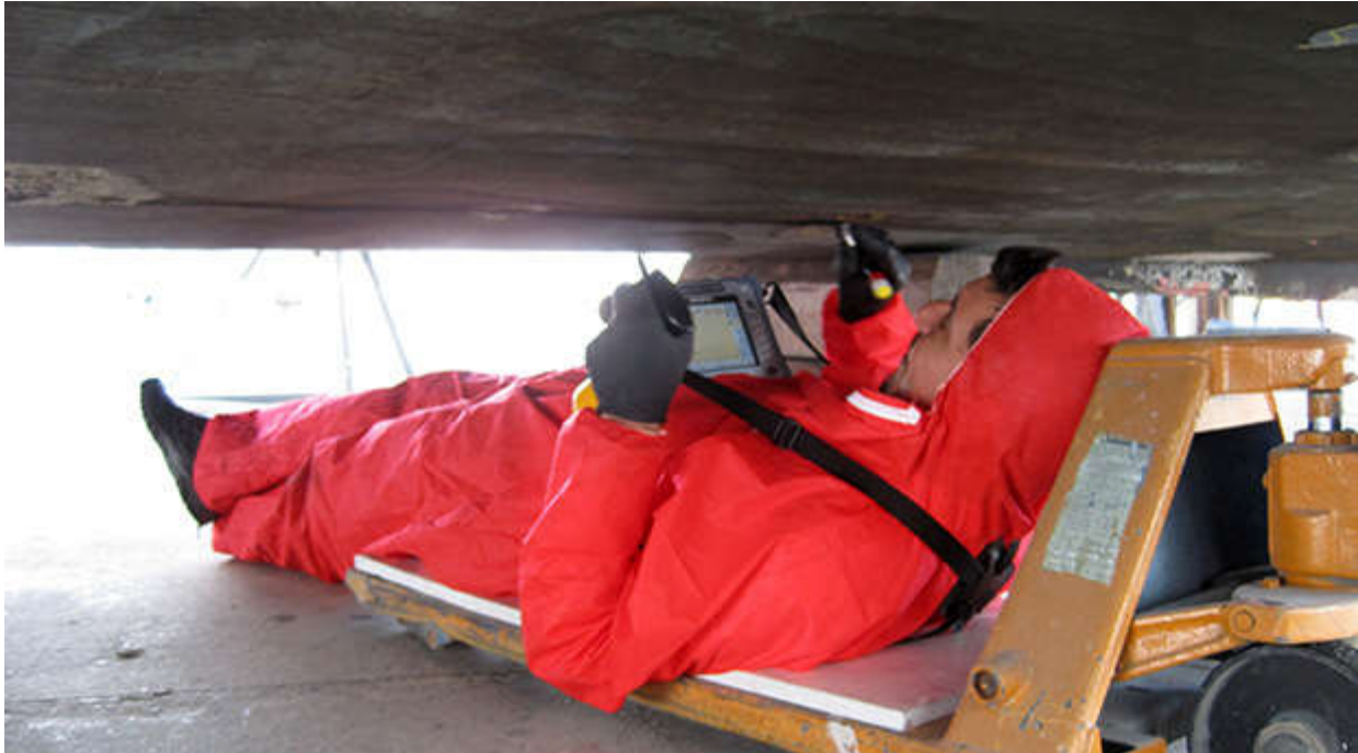
Cem Baykent performs ultrasonic testing of composite boats and spars using the EPOCH 650 flaw detector
