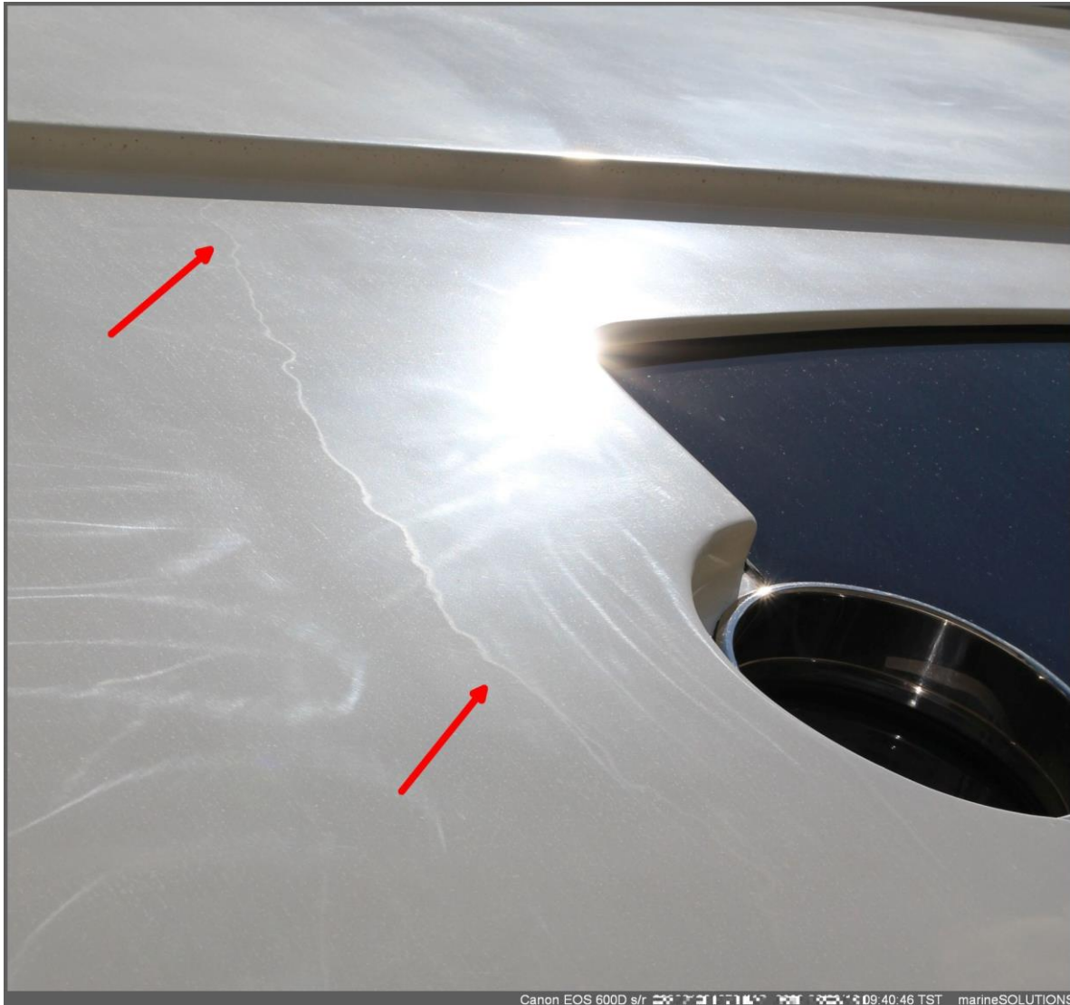
Transition mark around the port master cabin window – photo not altered.
