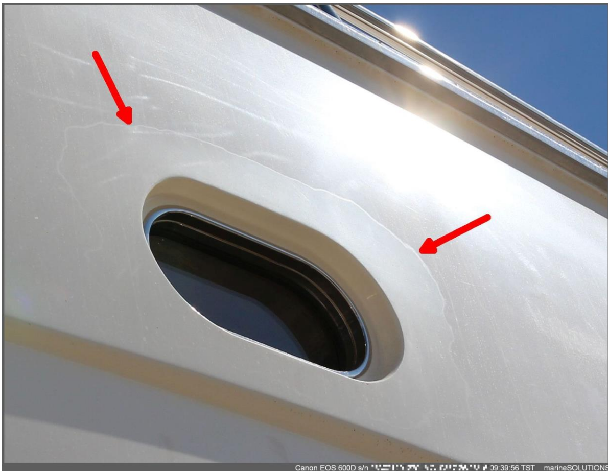
Transition marks around one of the portholes – photo not altered.
