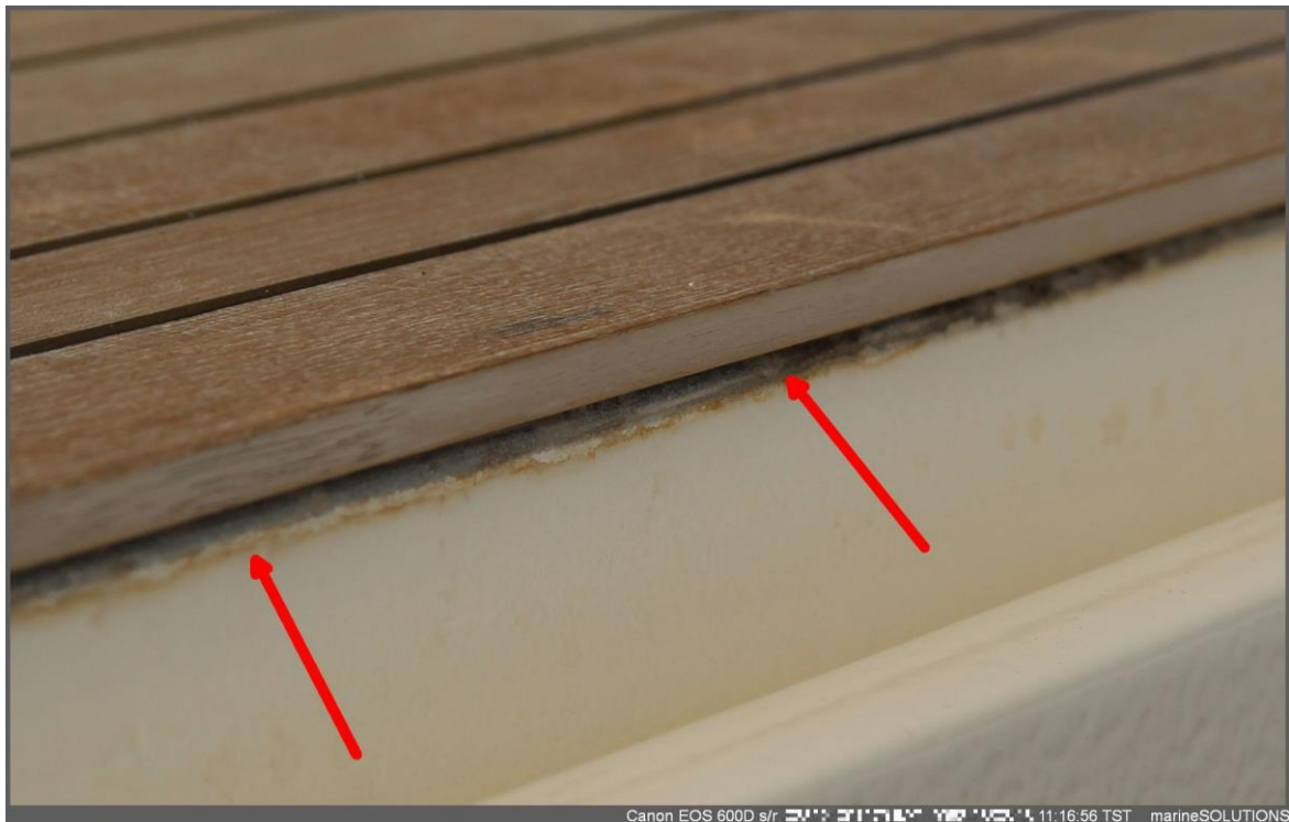
Detached teak plank around the engine room hatch at the cockpit.
