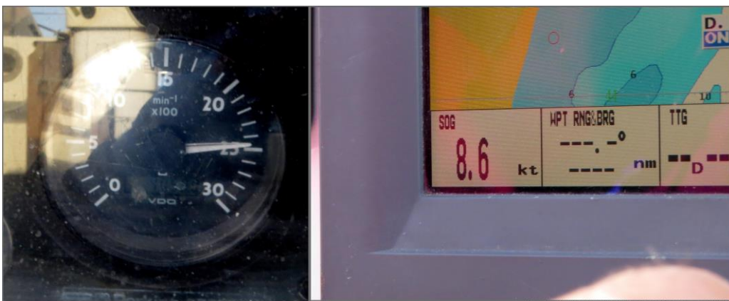
Above left: Maximum revs at full throttle. Above right: Maximum speed over ground at full throttle.
