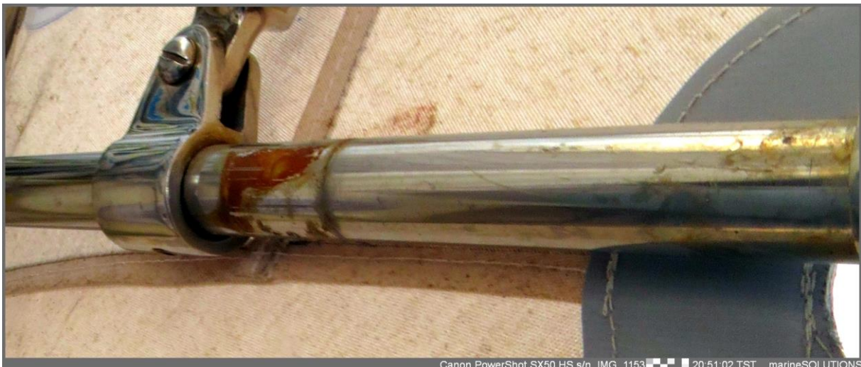
Above: Spray hood frame's rusted sections
