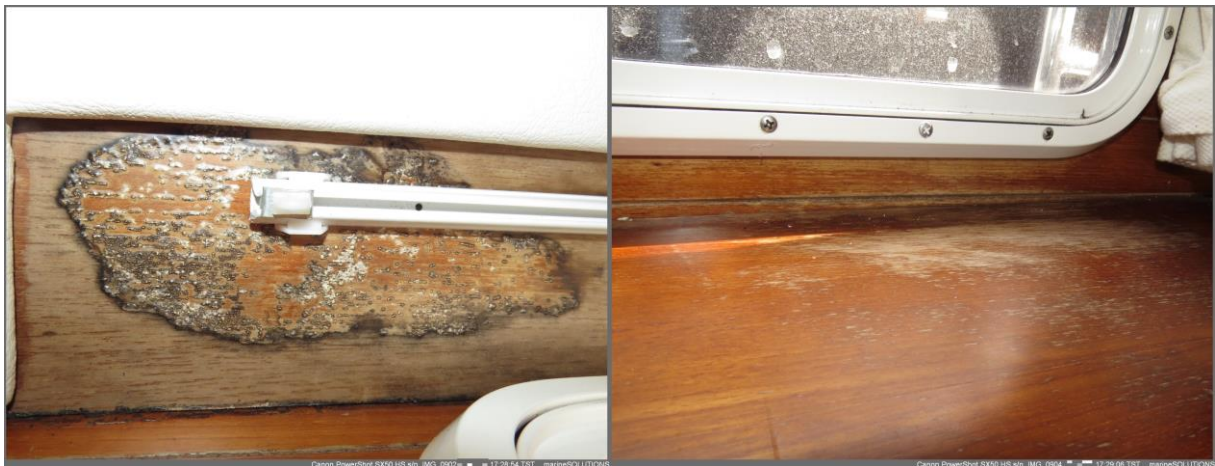
Above: Damaged veneer and varnish around the starboard porthole of the saloon
